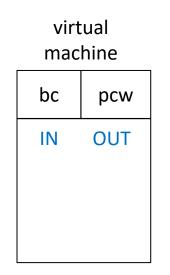
In the IN port, the parent of this VM provided a buffer capability bc for an opened file. The READ(IN) command within the virtual machine calls READ\_FILE(bc) on seeing that the type of the IN capability is for an open file buffer.
