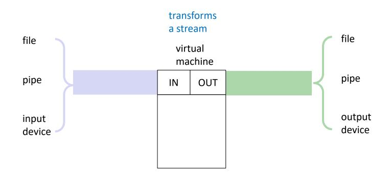
Streams allow great flexibility in constructing pipelines of virtual machines
