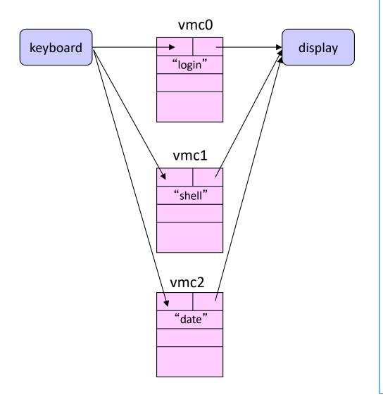
When the OS is started it creates a "login" VM (vmc0) attached to keyboard and display. When a user successfully types a user name and password, login creates a "shell" VM (vmc1) and goes to sleep.
