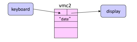
Each arrow represents a capability. Here the IN port of vmc2 contains a capability for a keyboard. The OUT port contains a capability for the display.
