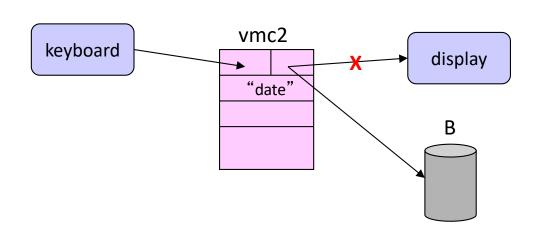
By default, a new VM inherits the standard IN and OUT of its parent.
