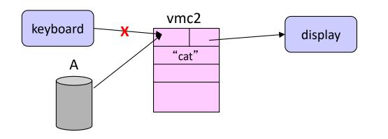
"cat" is a program that copies its input directly to its output. Here the user, with the notation "<A", has directed that a capability for file A be placed in IN, replacing the keyboard capability.
