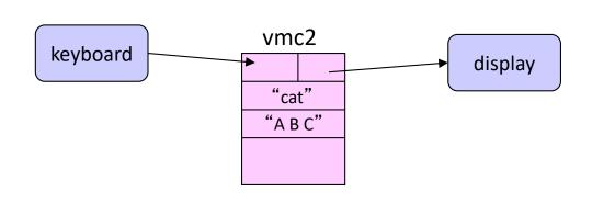
"cat" can also concatenate (string together) a series of files specified as arguments. In this case the code of "cat" ignores its IN and instead opens the files A, B, C by calling the file manager. It then reads them in turn, copying their contents to OUT, which is the display.
